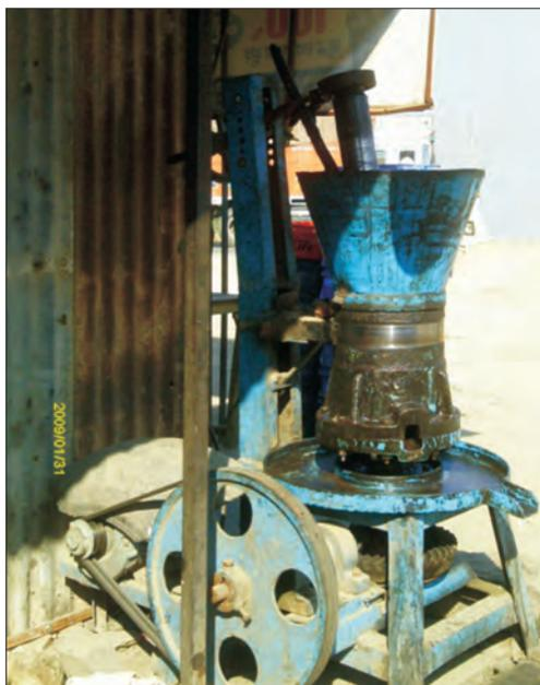
**Fig. 6.** In a big village of Rajasthan (Kharwa) Electric oil crusher machines are generally seen, which usually crush oil from the seeds brought by the farmers
