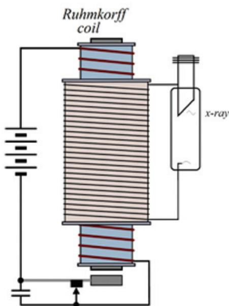
**Fig. 5.** Schematic diagram of X-ray apparatus using a Ruhmkorff's coil as a high voltage source as was used by Roentgen.
