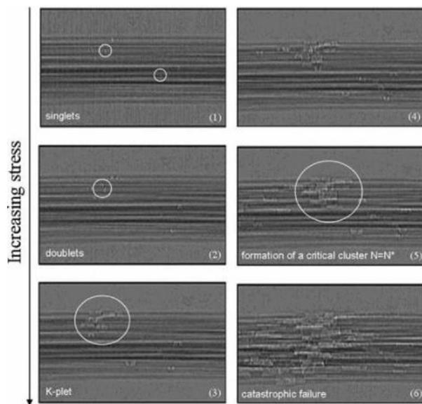
Fig. 1. Sequence of fiber failures in a unidirectional composite under axial tension (Aroush *et al.*, 2006)
