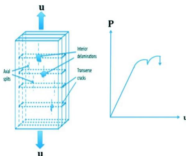
Fig. 8. Schematic illustration of multiple transverse cracking, axial splits and interior delamination as subcritical mechanisms in a cross-ply composite laminate. The load-displacement response under prescribed displacement is illustrated to the right
