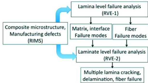
**Fig. 9: A roadmap for failure analysis of composite laminates**
