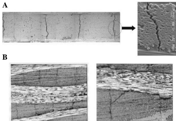
**Fig. 6. Multiple cracking in a laminate (A) and in a woven fabric composite (B)**
