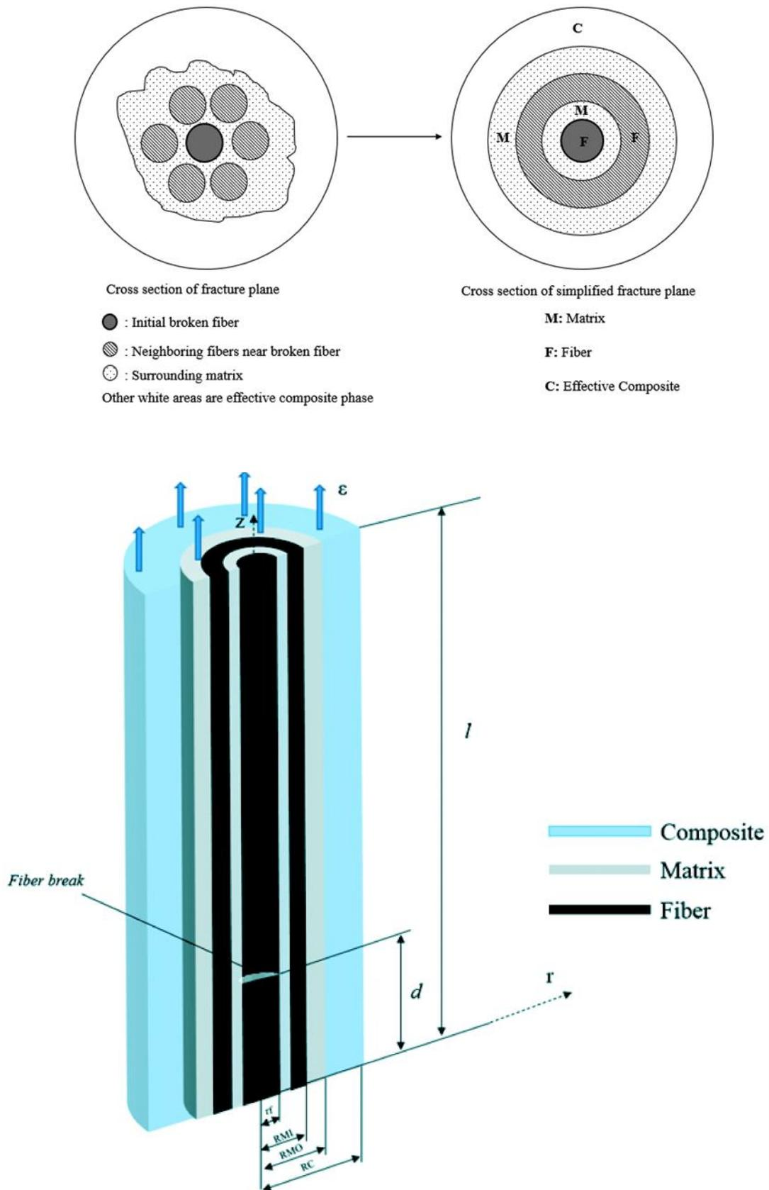
Fig. 7. The five-cylinder axisymmetric model for analysis of local failure from an initially broken fiber
