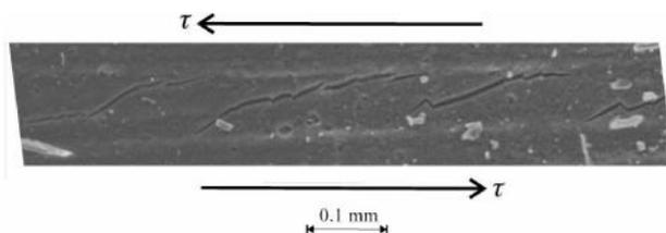
Fig. 5. Shear failure (From Redon, 2000)
