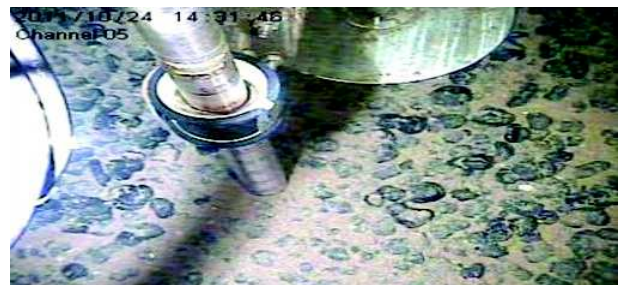
Fig. 7: Deep-sea soil tester at 5462m in CIOB
