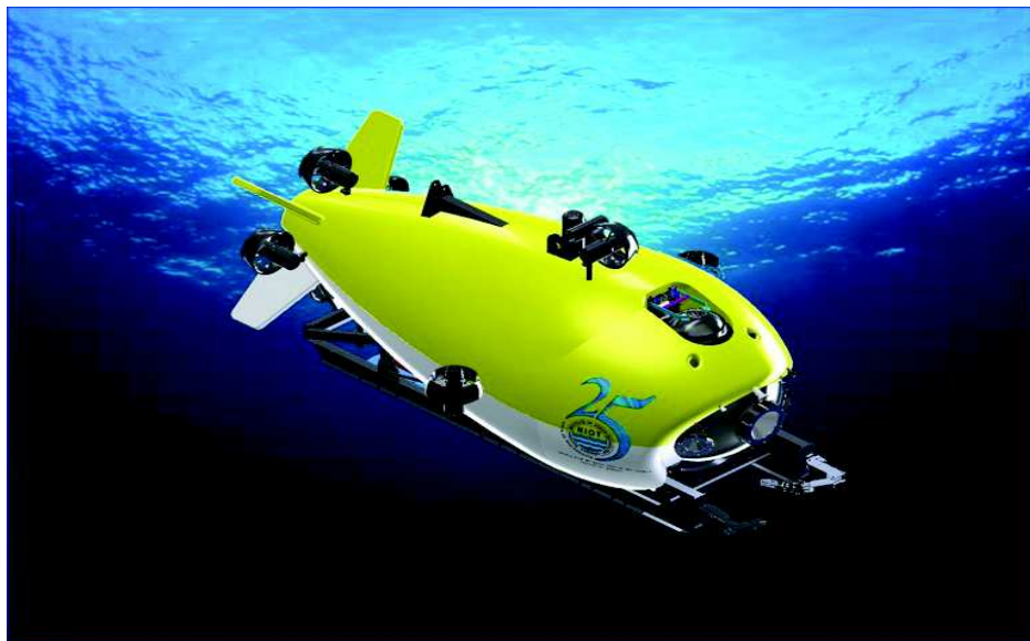
Fig. 15: Conceptual model of Deep-sea Manned-submersible-Matsya 6000
