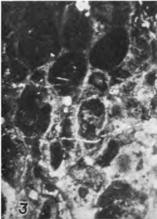
FIGS. 1-4 : (All Figures are from thin sections, plane polarised light). 1, Bedded massive phosphorite, showing infilled parallel joint planes, \times 40 ; 2, Bedded phosphorite showing the band of spherulites in the phosphate groundmass, \times 30 . 3, Phosphate pellets with anisotropic phosphate rims in anisotropic phosphate groundmass relatively free from detrital matter, \times 30 ; 4, Concentric-layered phosphate pellets occurring in a phosphate rich band associated with siltstone, \times 30 .
