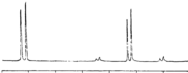
FIG 1 ^{31}\text{P}\{^1\text{H}\} NMR spectrum of [\text{PBu}_3\text{ClPd}(\mu\text{-Cl})_2\text{PtCl}(\text{PBu}_3)] in \text{CDCl}_3
