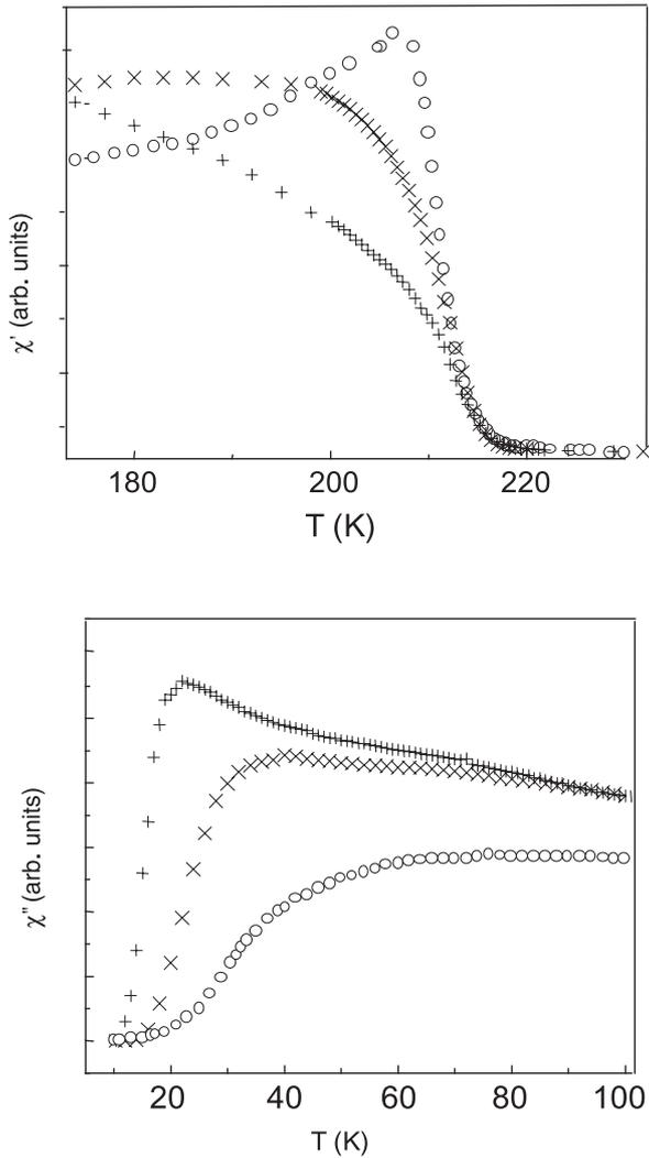
**Figure 2:** The real ( $\chi'$ ) and imaginary ( $\chi''$ ) components of ac susceptibility data measured in an applied field of 40 A/m (o), 400 A/m (x), and 1600 A/m (+) with 80 Hz frequency for  $a\text{-Fe}_{86}\text{Mn}_4\text{Zr}_{10}$  alloy.
