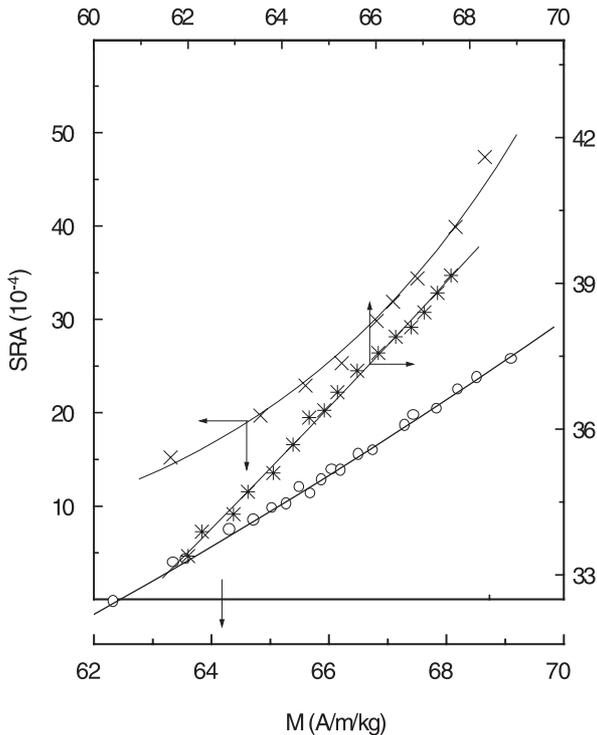
**Figure 9:** The relation between spontaneous resistive anisotropy and magnetization at different temperatures 4.2 K (o), 100 K (\*) and 200 K (x) for a- $\text{Fe}_{86}\text{Mn}_4\text{Zr}_{10}$  alloy
