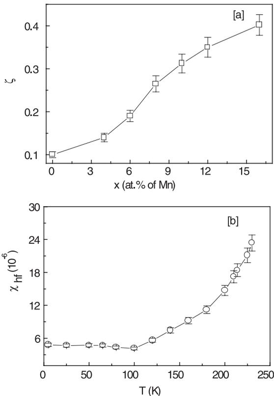
**Figure 6:** (a) The local magnetic anisotropy constant as a function of Mn concentration for  $a\text{-Fe}_{90-x}\text{Mn}_x\text{Zr}_{10}$  alloys and (b) the high-field susceptibility as a function of temperature for  $a\text{-Fe}_{82}\text{Mn}_8\text{Zr}_{10}$  alloy.
