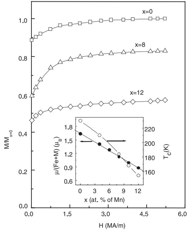
**Figure 4:** The magnetic isotherms for  $a\text{-Fe}_{90-x}\text{Mn}_x\text{Zr}_{10}$  alloys. The magnetization axis is normalized with respect to the magnetization values at 5.2 MA/m for  $x=0$ . Inset: The composition dependent average magnetic moment and Curie temperature of  $a\text{-Fe}_{90-x}\text{Mn}_x\text{Zr}_{10}$  alloys
