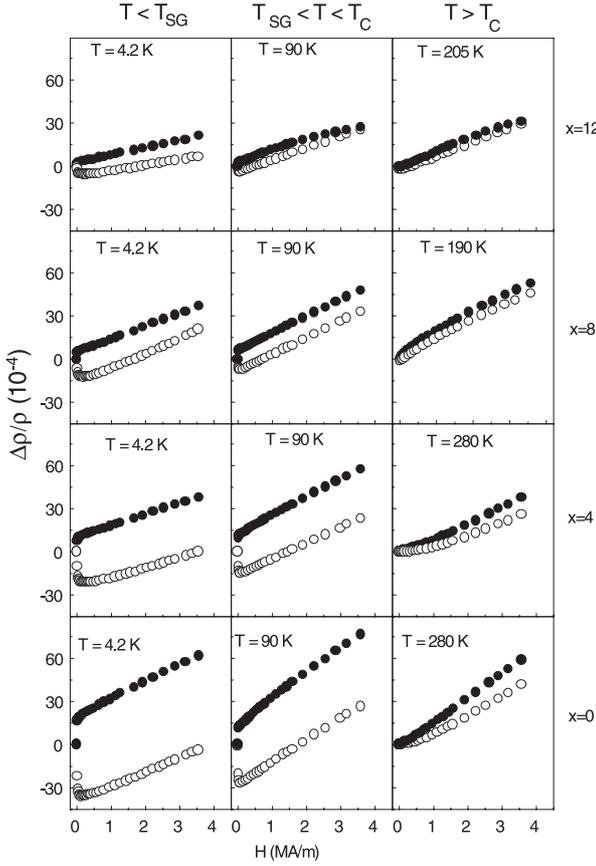
**Figure 7:** Longitudinal (●) and transverse (○) magnetoresistance as a function of field for  $a\text{-Fe}_{90-x}\text{Mn}_x\text{Zr}_{10}$  alloys obtained at different temperatures:  $T < T_{SG}$ ,  $T_{SG} < T < T_C$  and  $T > T_C$
