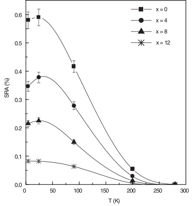
**Figure 8:** Spontaneous resistive anisotropy as a function of temperature for  $a\text{-Fe}_{90-x}\text{Mn}_x\text{Zr}_{10}$  alloys
