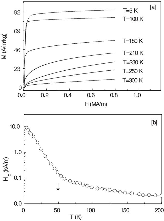
**Figure 5:** (a) Magnetic isotherms at different temperatures and (b) temperature dependent coercivity for  $a\text{-Fe}_{82}\text{Mn}_8\text{Zr}_{10}$  alloy.
