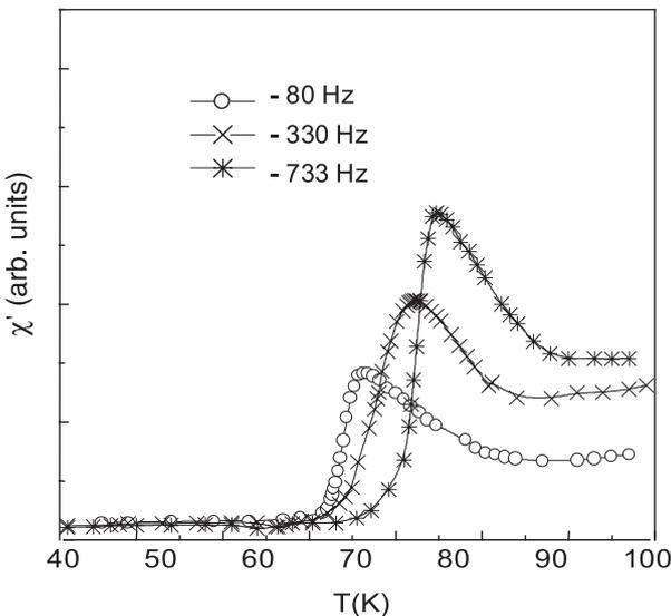
**Figure 3:** The imaginary ( $\chi''$ ) component of ac susceptibility data measured in an applied field of 1600 A/m with different frequencies 80 Hz (-o-), 330 Hz (-x-) and 733 Hz (-\*-) for  $a\text{-Fe}_{30}\text{Mn}_{10}\text{Zr}_{10}$  alloy
