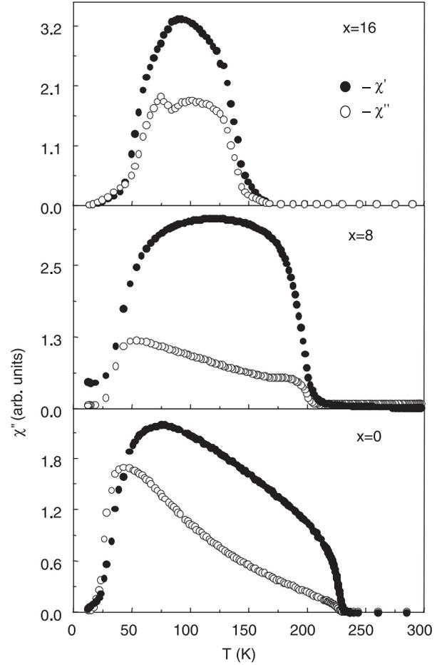
**Figure 1:** The real ( $\chi'$ ) and imaginary ( $\chi''$ ) components of ac susceptibility data measured in an applied field of 1600 A/m with 80 Hz frequency for a-Fe<sub>90-x</sub>Mn<sub>x</sub>Zr<sub>10</sub> ( $x = 0, 8, 16$ ) alloys
