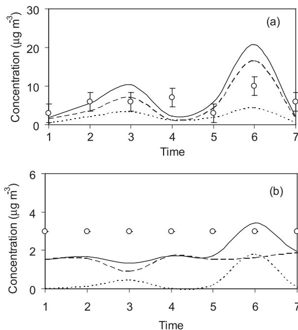
**Figure 5:** Comparison of predicted and observed  $\text{NO}_x$  concentrations in summer season at (a) Fire Office and (b) Sriharipuram in Visakhapatnam bowl area. GPM -----; CALINE3 - - - - -; Cumulative concentrations ——— Observed O. Errors bars are standard deviations of the observed values
