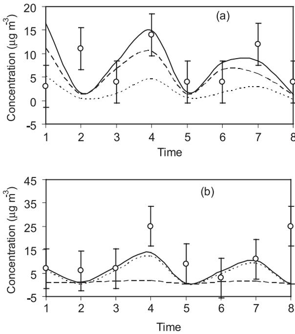
**Figure 6:** Comparison of predicted and observed  $\text{NO}_x$  concentrations in winter season at (a) Gajuwaka and (b) Karasa in Visakhapatnam bowl area. GPM -----; CALINE3 -----; Cumulative concentrations ———— Observed O. Errors bars are standard deviations of the observed values
