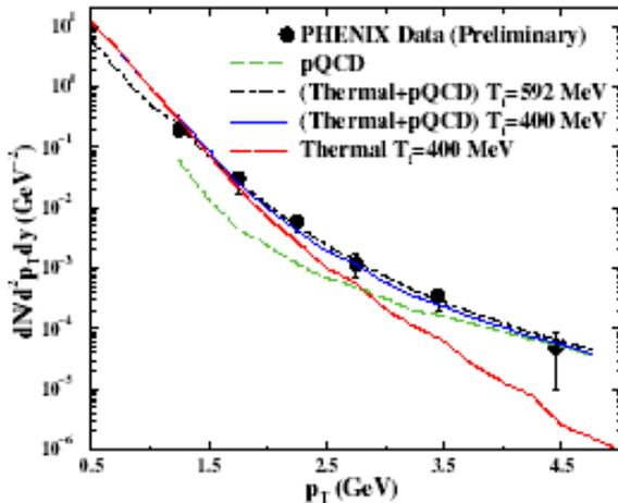
Fig. 8: Direct photon spectra at RHIC energies measured by PHENIX Collaboration. Dashed line indicates hard photons from NLO pQCD calculations. Solid (dot-dashed) line depicts the total (pQCD + thermal) photon yield obtained from QGP initial state with  $T_i = 400$  MeV and  $n = 0.2/m/c$  ( $T_i = 592$  MeV  $n = 0.15$  fm/c). In medium effects on hadrons are included (ignored) in the results shown by solid (dot-dashed) line.
