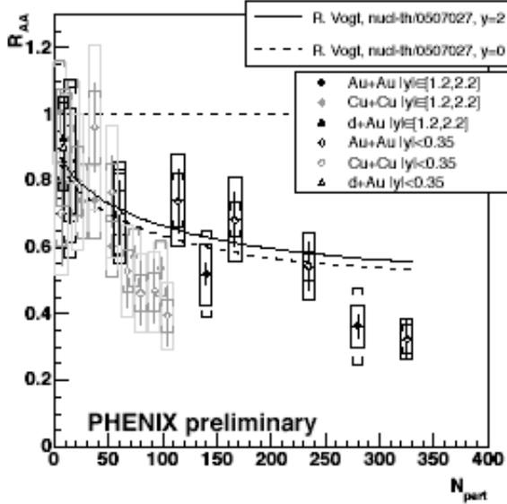
Fig. 7:  $J/\psi$  nuclear modification factor as a function of the number of participant, compared to  $R_{AA}$ . Vogt predictions for the normal nuclear absorption. Vertical bars are statistical errors, brackets are point to point systematics and boxes are global systematics.
