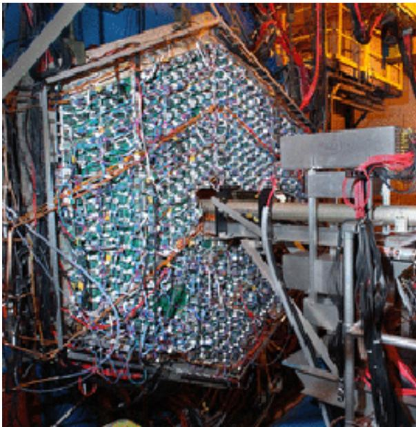
**Fig. 9:** View of the preshower plane of STAR, PMD from the RHIC tunnel side
