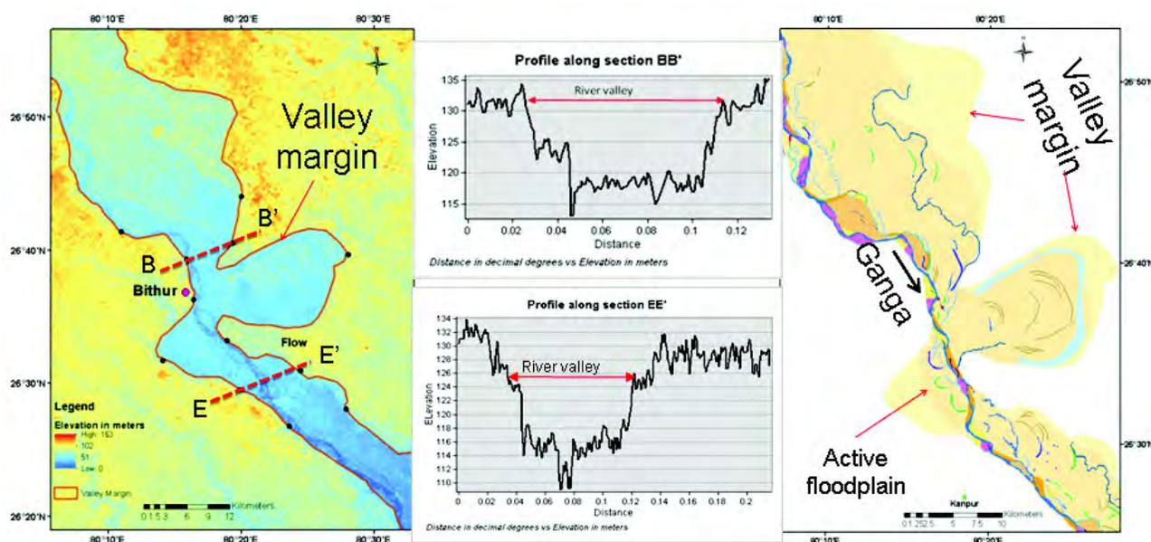
Fig. 10: Defining 'River space' as active floodplains and valley margin for a stretch of the Ganga river around Bithur (Kanpur); valley margin was mapped from SRTM-DEM and active floodplain was delineated from the satellite image (GRBEMP, 2010)
