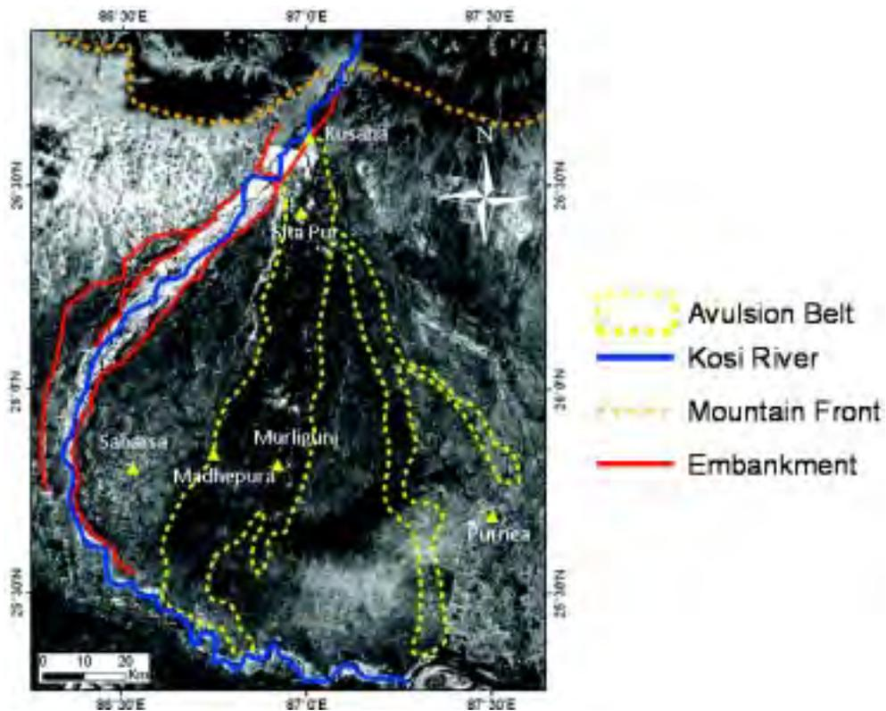
Fig. 5: The August 2008 avulsion of the Kosi River caused by the breach of the eastern embankment at Kusaha in Nepal. The avulsion belt reoccupied one of the paleochannels of the Kosi and 80-85% of the total flow found its way into this course
