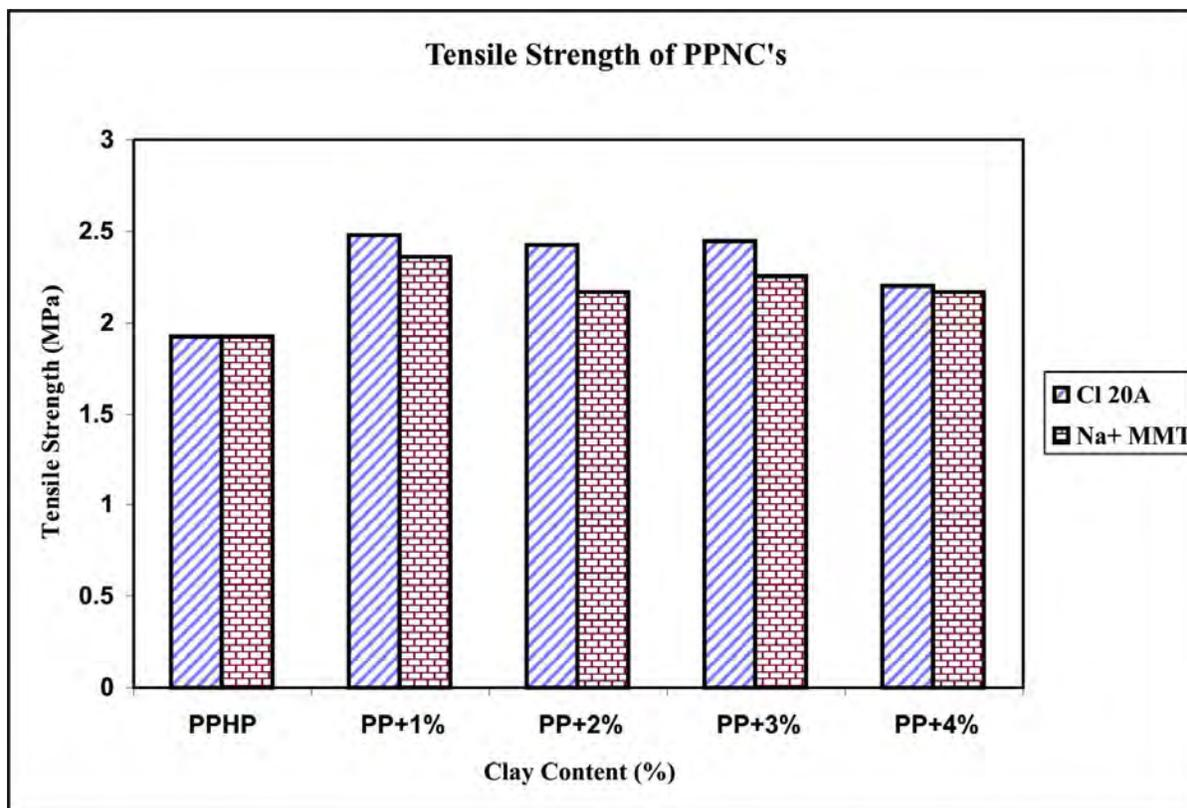
Fig. 6: Tensile Strength vs Filler conc Histogram of PPNCs
