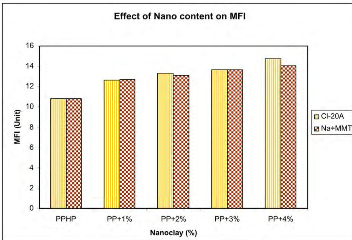
Fig. 5: Melt Flow Index vs Filler conc Histogram of PPNCs
