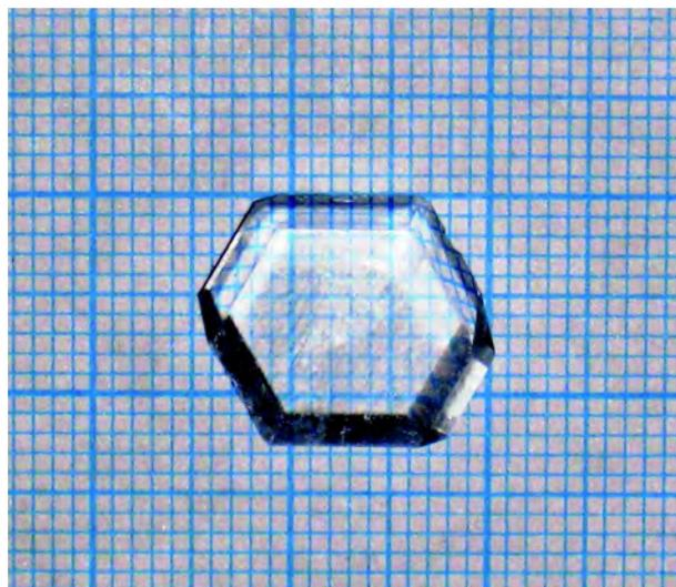
Fig. 1: Photograph of as-grown GPI crystal
