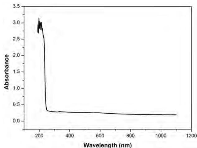
**Fig. 4: Optical absorption spectrum of GPI**
