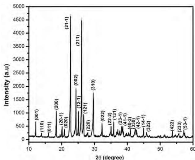
Fig. 2: Powder XRD pattern of GPI
