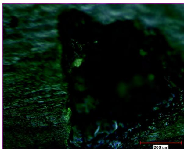
Fig. 8: Optical micrograph of the CMST crystal surface after passing laser beam of 16.7 mJ for 30 s time
