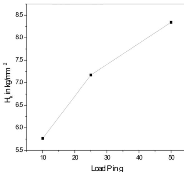
Fig. 6: Variation of Knoop hardness  $H_k$  with load
