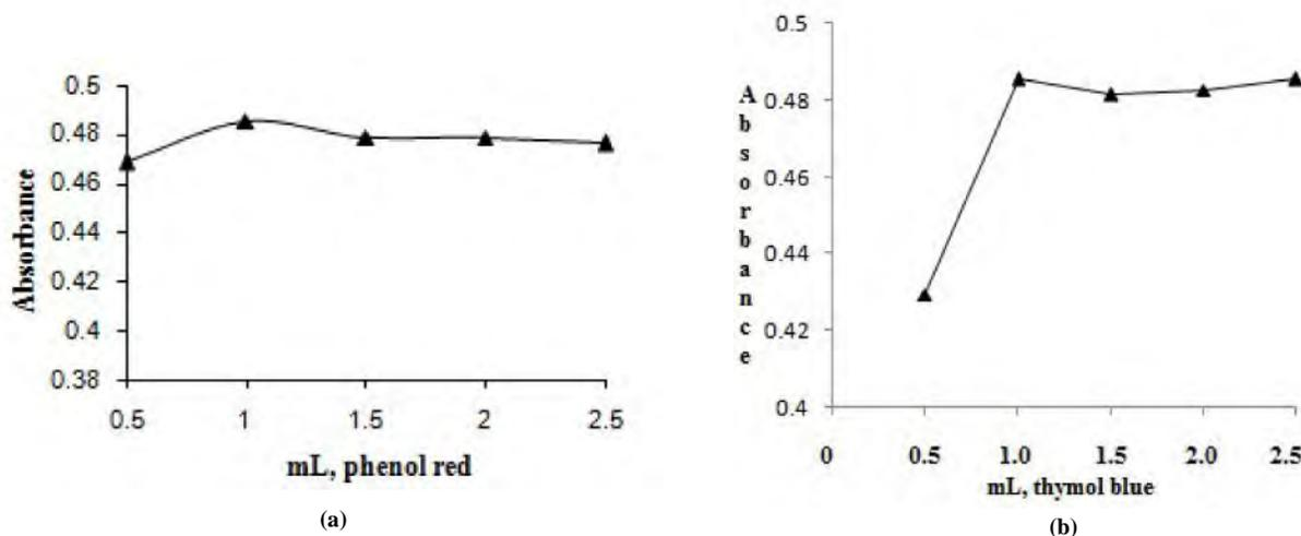
Fig. 2: Effect of reagent volume: (a) 0.01% Phenol red ( $0.2 \mu\text{g ml}^{-1}$  PYL) in method A and (b) 0.01% Thymol blue ( $0.4 \mu\text{g ml}^{-1}$  PYL) in method B
