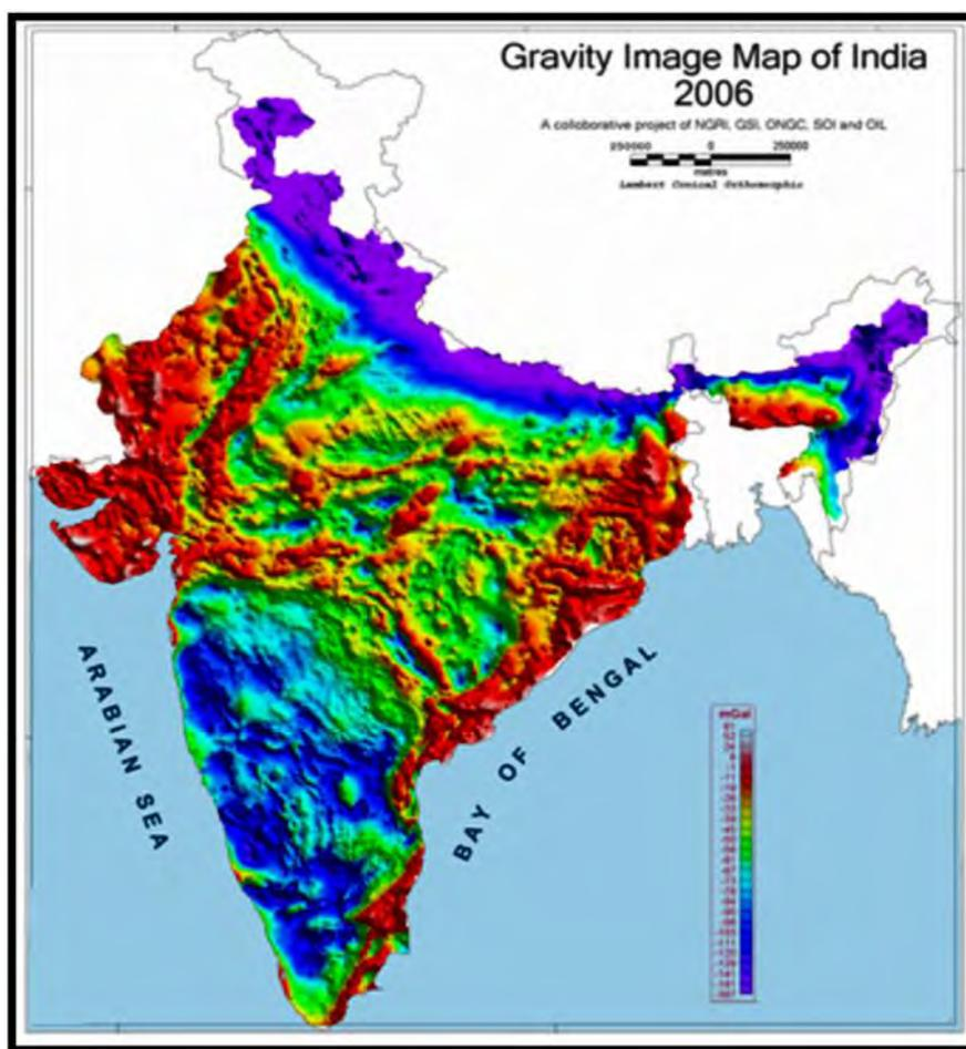
Fig. 2: Bouguer Gravity Anomaly Map of India depicting nature of anomalies in the different parts of India. High (red) and low (blue) values of gravity anomalies indicate high and low subsurface density distributions respectively. Source: Gravity Map Series of India-2006
