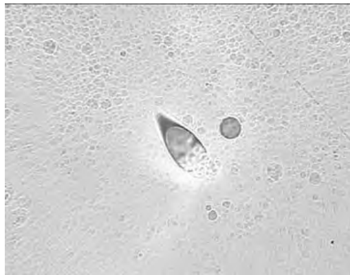
Fig. 4: Heavy ion track on CR-39 at Hanle
