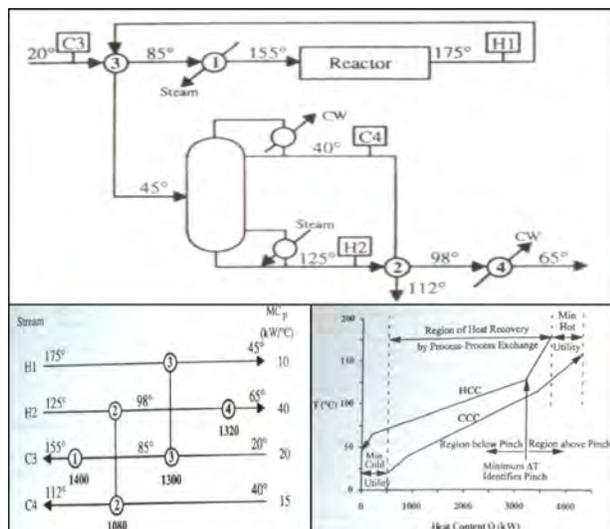
**Fig. 2: Concepts of pinch technology in distillation process**
