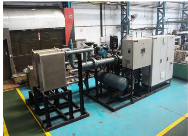
Fig. 6: Indigenously developed 100 kW<sub>e</sub> power skid
