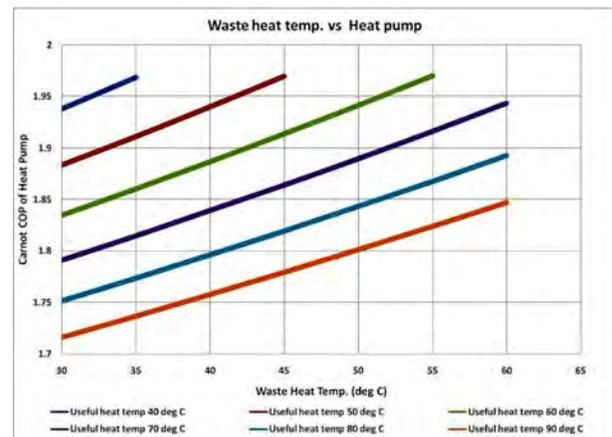
Fig. 3: Carnot COP of absorption heat pump (Type 1)
