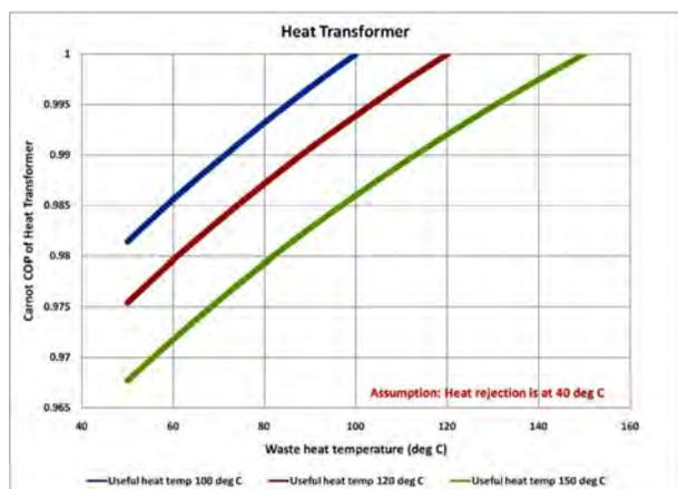
Fig. 4: Carnot COP of heat transformer (Type 2)
