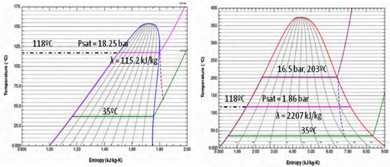
Fig. 5: TS diagram of R245fa and water (NIST 2013)
