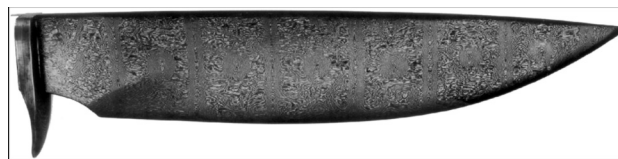
Fig. 1 Reconstructed wootz steel blade [reproduced with permission from Verhoeven et al. (1998, pp. 58–64) © 1998 The Minerals, Metals & Materials Society]
