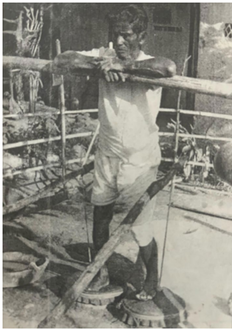
Fig. 8 A bellowsmen operating the bellows during an iron smelting process at Kakching. (Photo source: Gourachandra, 2002, p. 55)
