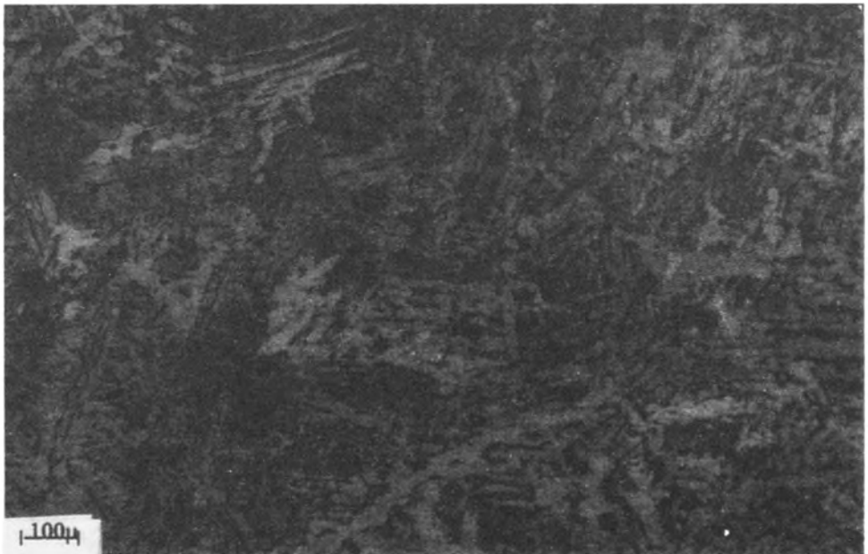
Fig. 3 : Micro structure in the longitudinal section showing a Widmanstätten structure.
