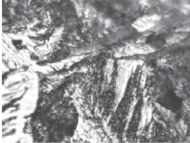
**Fig. 23.** Micrograph revealing bainitic Structure in the matrix, 1000X
