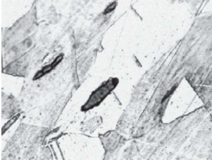
**Fig. 18.** Micrograph showing elongated lead particles, slip bands, 1500X
