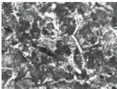
**Fig. 24.** Cracked corroded region, 200X
