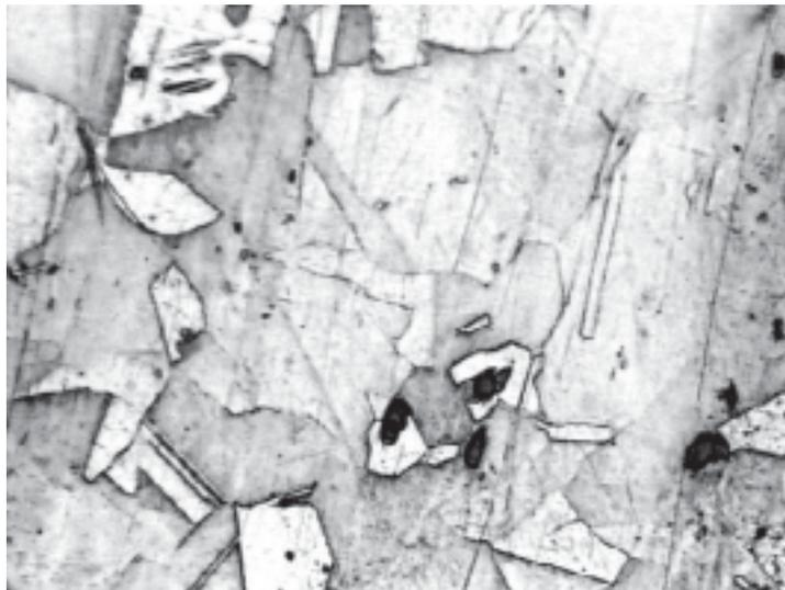
**Fig. 19.** Micrograph showing twin bands, 1000X
