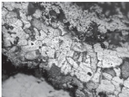
**Fig. 22.** Iron artefact in different stages of corrosion 200X
