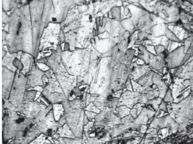
**Fig. 20.** Micrograph illustrating twin bands, globular lead particles and equiaxed grain structure, 200X
