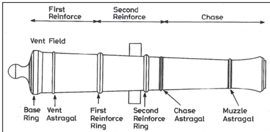
Fig. 2. Schematic diagram showing the various parts of typical cannon
