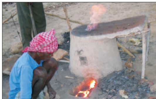
Fig. 2. Iron Smelting in Modern Agaria Furnace, Singarauli, Madhya Pradesh
