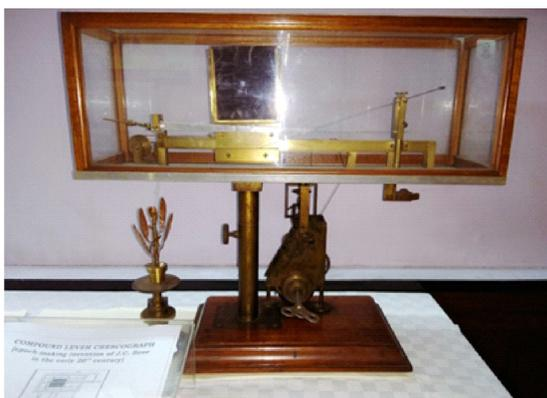
**Fig. 2.** Compound Lever Crescograph– An apparatus invented by JC Bose in early 20<sup>th</sup> century, on display at the Bose Museum in Kolkata.
