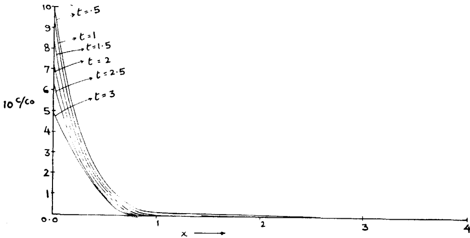
FIG. 3. The variation of C/C_0 against the distance. u = 6 cm/min, D = 0.6 cm 2 /min.
