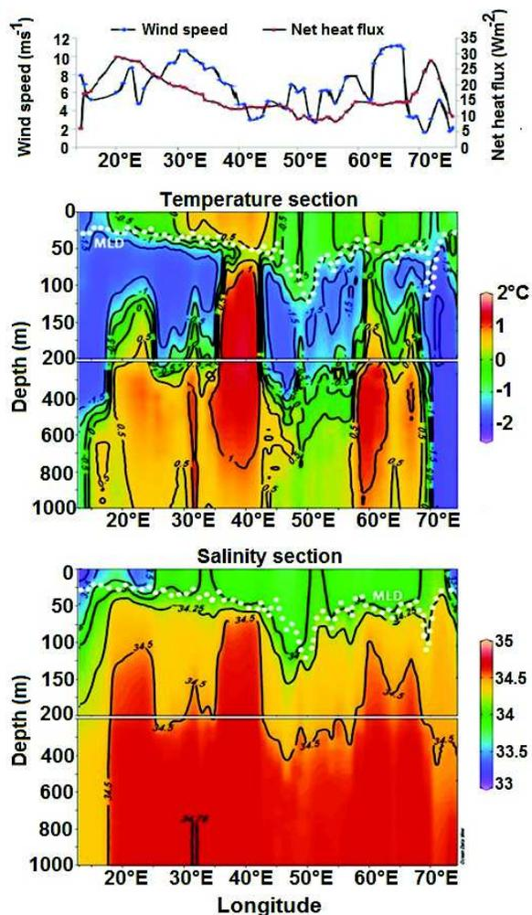
Fig. 4: Vertical temperature and salinity structures prepared from XCTD observations recorded during 19<sup>th</sup>-25<sup>th</sup> February, 2013. Mixed layer depth (represented by white dots) has been calculated as the depth where density change of  $0.03 \text{ kgm}^{-3}$  is encountered from surface value (Dong *et al.*, 2008). Surface meteorological parameters were derived from ECMWF interim forecast (Berrisford *et al.*, 2011)
