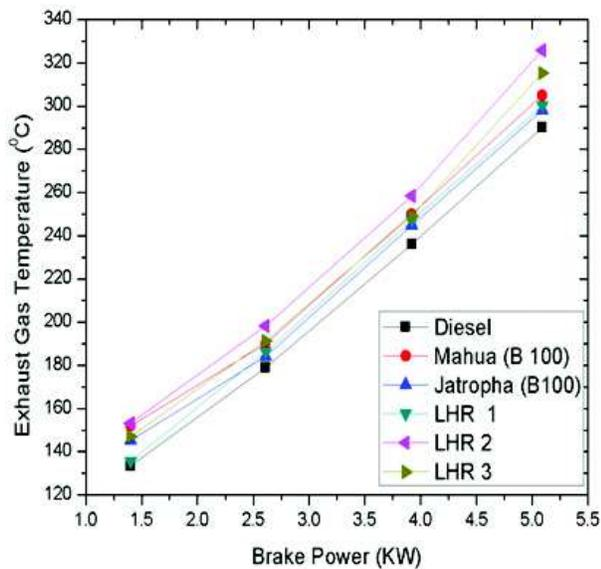
Fig. 8: Variation of exhaust gas temperatures with brake power
