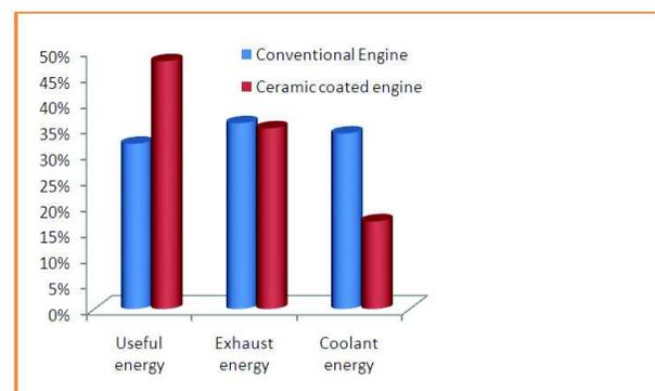
**Fig. 1: Comparison of conventional and ceramic coated engines (Buyukkaya and Cerit 2008)**
