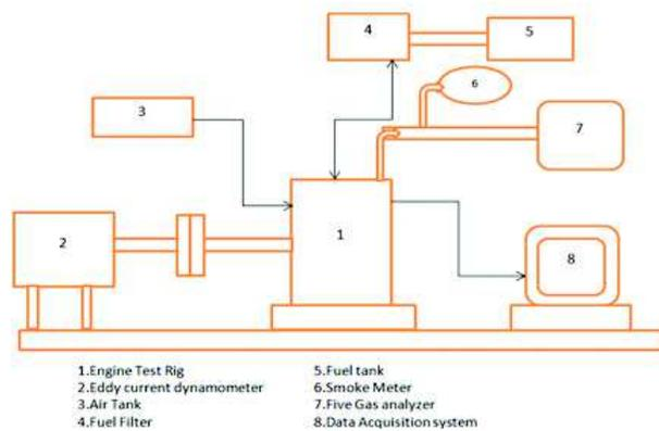
Fig. 5: Engine schematic diagram
