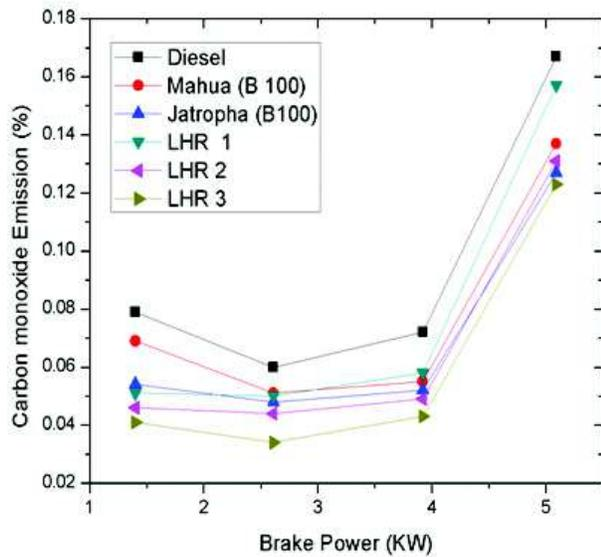
Fig. 10: Variation of Carbon monoxide emission with brake power
