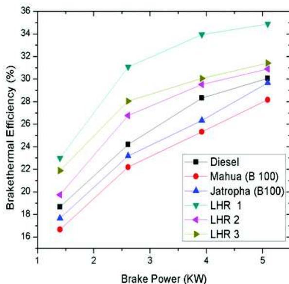
Fig. 6: Variation of brake thermal efficiency with brake power
