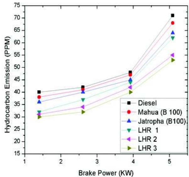
Fig. 9: Variation of hydrocarbon emission with brake power
