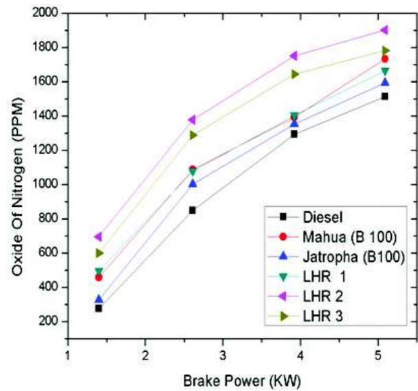
Fig. 11: Variation of oxides of nitrogen with brake power
