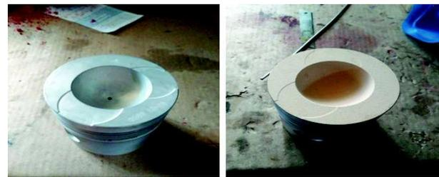
**Fig. 3: Snapshots of (a) uncoated baseline engine piston (b) 7%YSZ coated piston**
