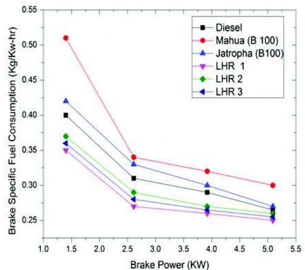
Fig. 7: Variation of brake specific fuel consumption with brake power
