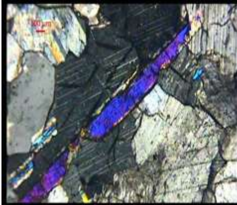
Fig.03: Photomicrograph of euhedral anhydrite lath in sparry calcite (calcite II) vein. TL, XN.
