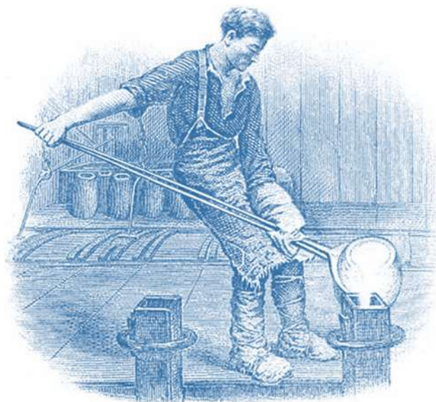
Fig. 13 Illustration of the crucible process for steelmaking. A worker is shown manipulating molten steel within a ceramic crucible using long tongs, demonstrating one of the earliest controlled methods of producing high-quality steel through localized melting and refining (Holappa 2019)
