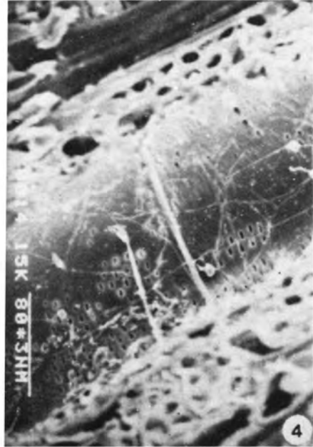
Figures 1-4 Scanning electron micrographs of sound and decayed sapwood of D. sissoo : 1 , TS of sound sapwood showing thick-walled, rigid cell wall structures; 2 , TS of decayed wood showing enzymatic softening of cell walls of fibres resulting in partial collapse of wall structures. Localised thinning, swelling and fragmentation of cell walls and clear distribution of hyphae in some wood elements; 3 , LS of sound sapwood showing medullary ray cells and fibres; 4 , LS of decayed sapwood showing dissolution of medullary ray cells, thinning of cell walls in some places and clear bore holes on wall structure ( b , bore hole; f , fragmentation; s , swelling; and t , thinning).
