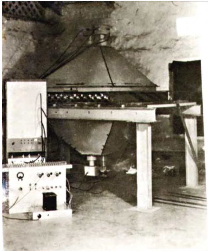
Fig. 1 The scintillator-lead-GM counter telescope used at great depths in KGF mines. A coincidence of pulses from PMTs viewing the two scintillators and the sandwiched GM counter array provided the signal with negligible background.
