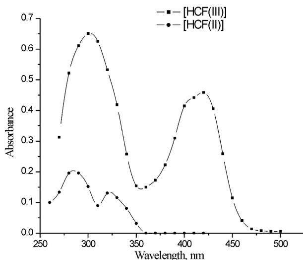
Fig. 1. Spectrum of HCF(III) and HCF(II) in  $0.1 \text{ mol dm}^{-3}$  NaOH at  $30^\circ\text{C}$
