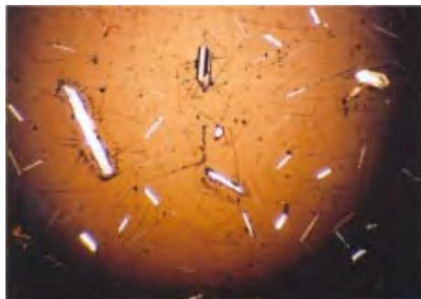
Fig. 2. Needle shaped crystals of Cysteic acid
