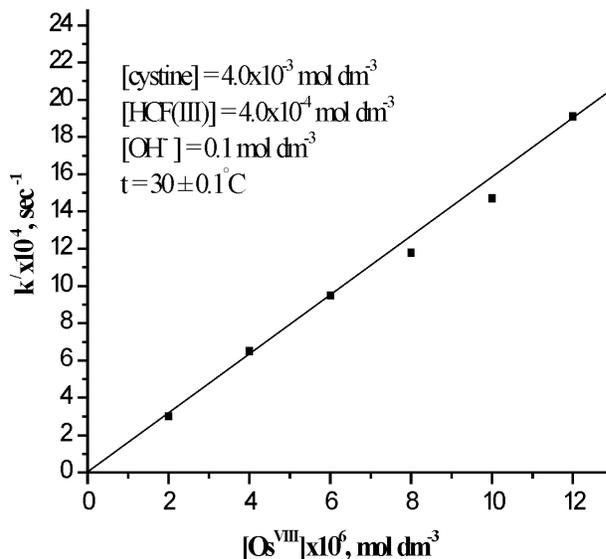
Fig. 4. Plot of  $k'$  versus  $[\text{osmium (VIII)}]$  (order with respect to  $[\text{osmium (VIII)}]$ )
