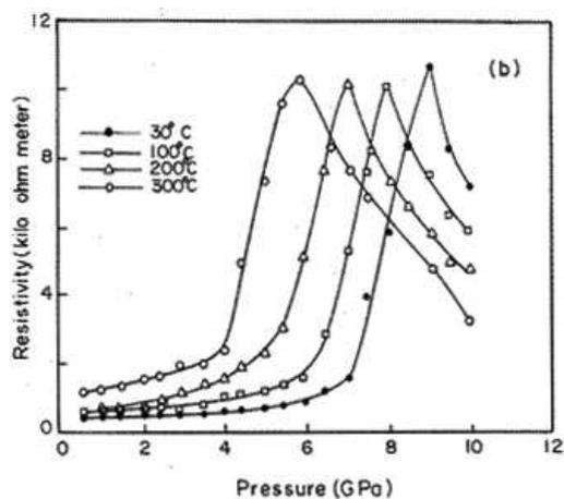
Fig. 1: Resistivity vs Applied Pressure at different temperatures for nano PbSe
