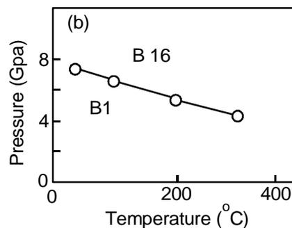
Fig. 2: Temperature-Pressure phase diagram of nano PbSe
