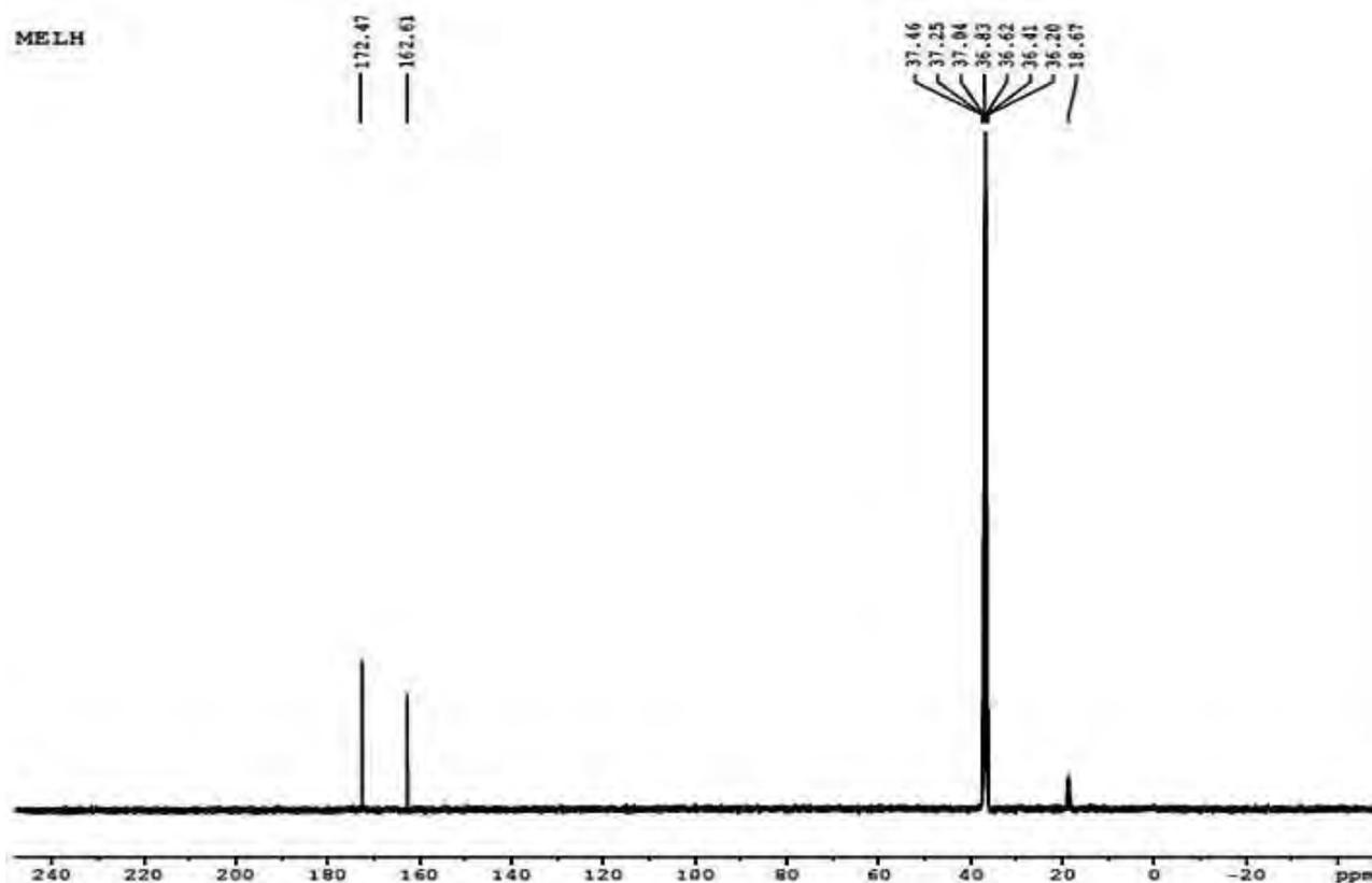
Fig. 4b: Carbon NMR spectrum of 2, 4, 6 triamino-1, 3, 5 triazine (melamine) crystal
