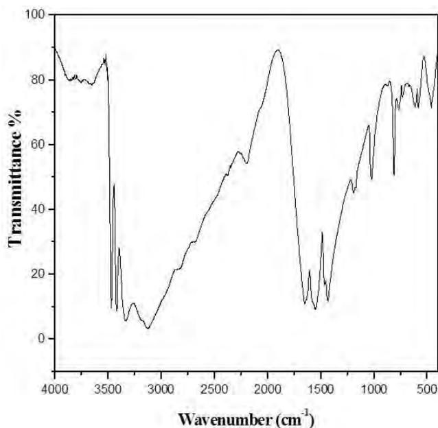
**Fig. 3: FTIR spectrum of 2, 4, 6 triamino-1, 3, 5 triazine (melamine) crystal**
