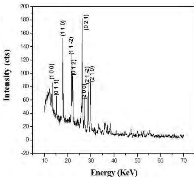
**Fig. 2: Powder XRD pattern of 2,4,6 triamino-1,3,5 triazine (melamine) crystal**
