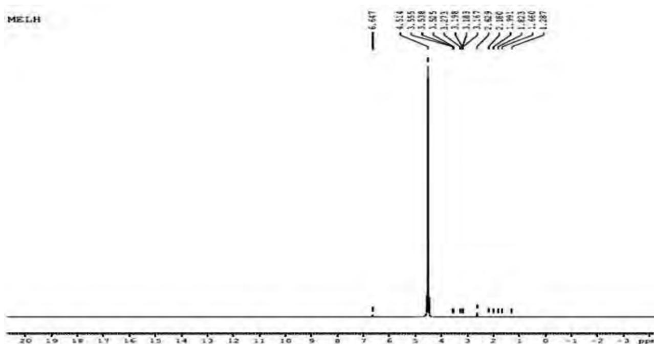
Fig. 4a: Proton NMR spectrum of 2, 4, 6 triamino-1, 3, 5 triazine (melamine) crystal
