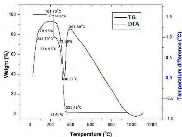
Fig. 5a: TG-DTA spectrum of 2, 4, 6 triamino-1, 3, 5 triazine (melamine) crystal
