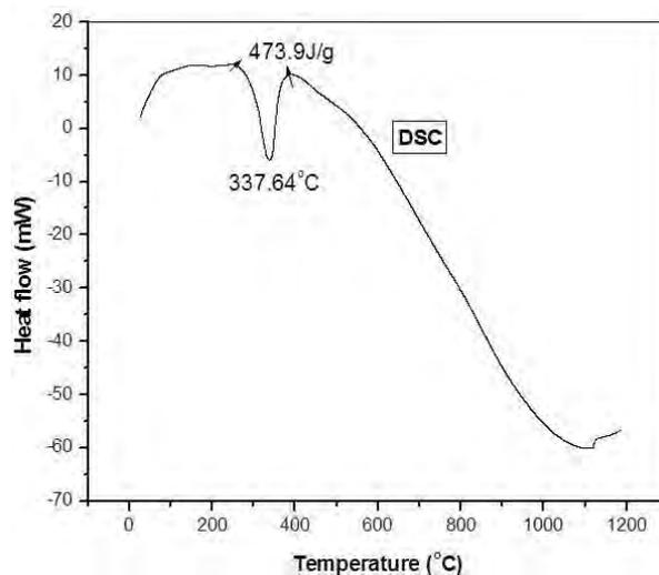
Fig. 5b: DSC spectrum of 2, 4, 6 triamino-1, 3, 5 triazine (melamine) crystal
