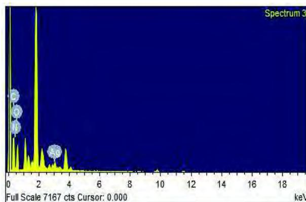
Fig. 7: EDS spectrum of silver nanoparticles (AgNps)
