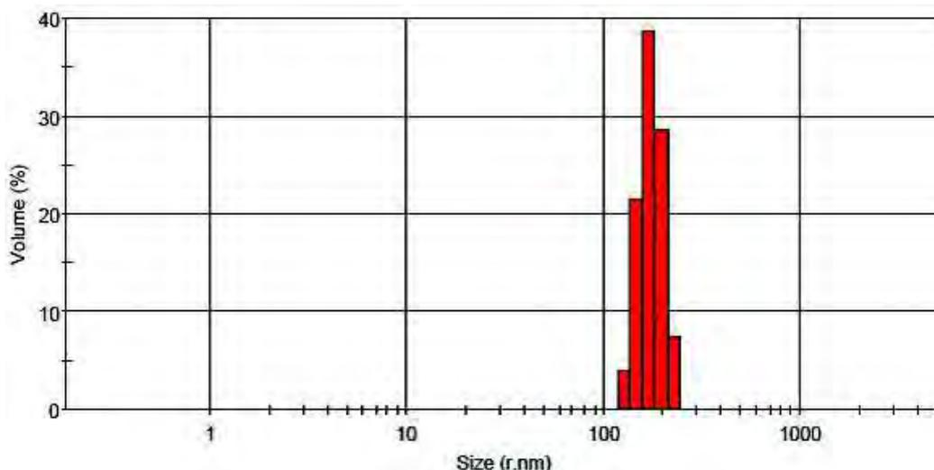
Fig. 8: Particle size distribution of AgNps with an average size of 176.4 nm
