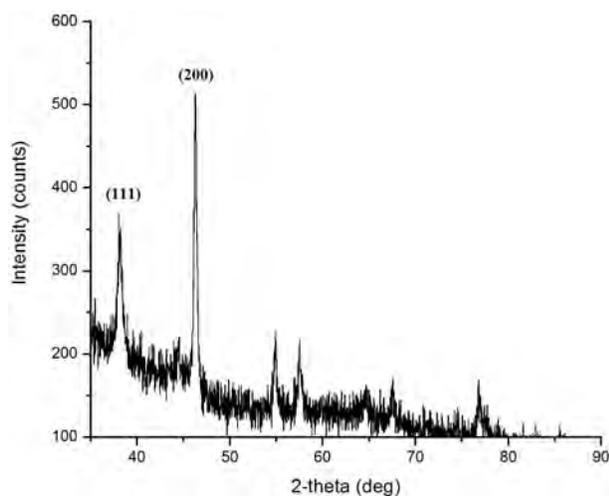
Fig. 5: X-Ray Diffraction patterns of AgNps showing peak indices and  $2\theta$  positions
