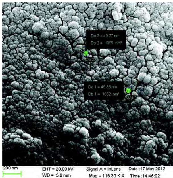
Fig. 6: SEM image of silver nanoparticles of average size of 40-45nm (scale bar corresponds to 200 nm)
