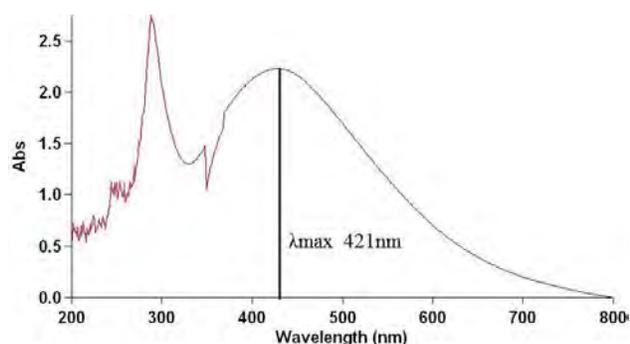
Fig. 2: UV-Vis spectrum of AgNps with maximum absorbance at 421 nm
