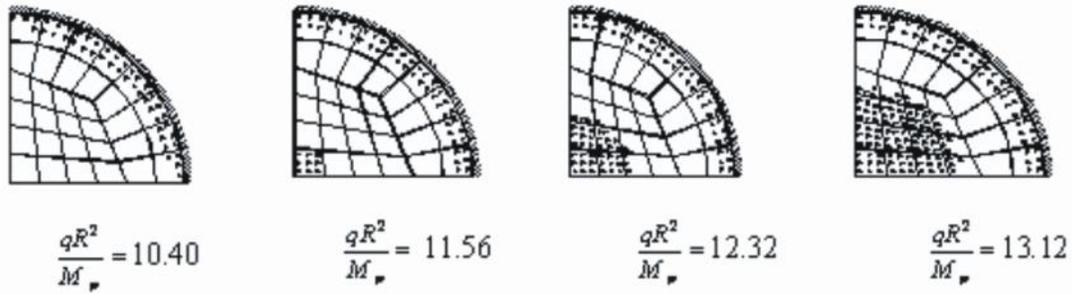
Fig. 3: Progress of plastic zone with load increments for  $d/h=20$ : Clamped circular plate with uniformly distributed load (HOST)
