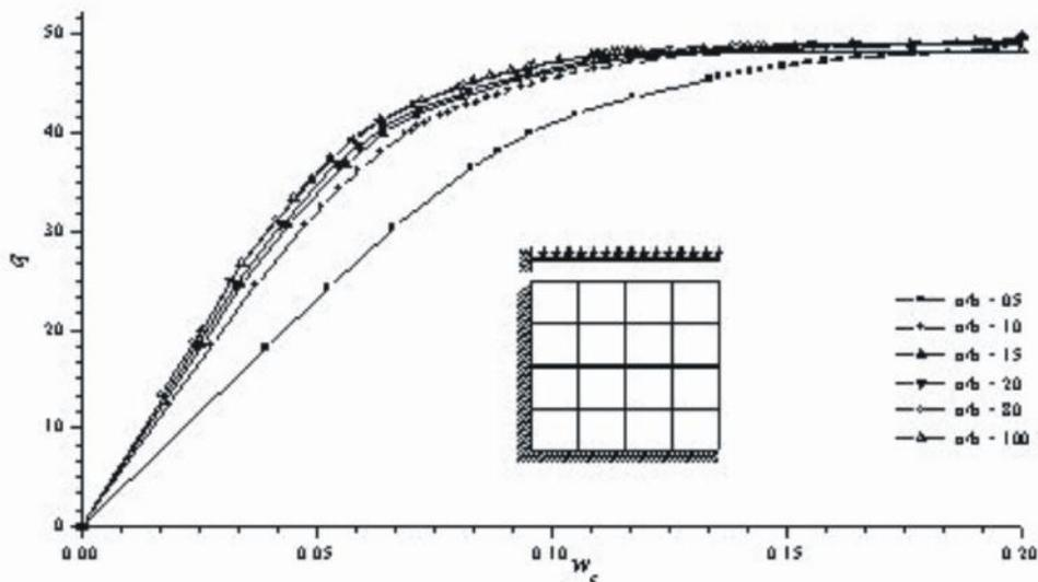
Fig. 5: Normalised load versus normalised central displacement for clamped circular plate with uniformly distributed load: Comparisons of different  $a/h$  ratios (HOST)
