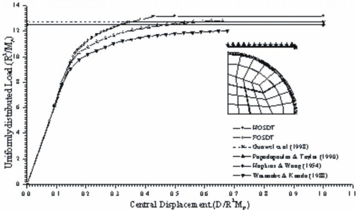
**Fig. 1: Normalised load versus normalised central displacement for clamped circular plate with uniformly distributed load: Comparisons of different formulations for d/h=100**
