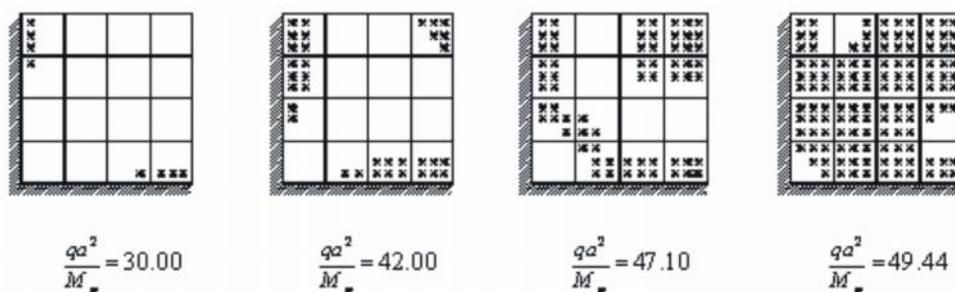
Fig. 6: Progress of plastic zone with load increments for a/h=30: Clamped circular plate with uniformly distributed load (HOST)
