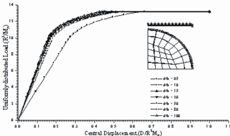
Fig. 2: Normalised load *versus* normalised central displacement for clamped circular plate with uniformly distributed load: Comparisons of different  $d/h$  ratios (HOST)
