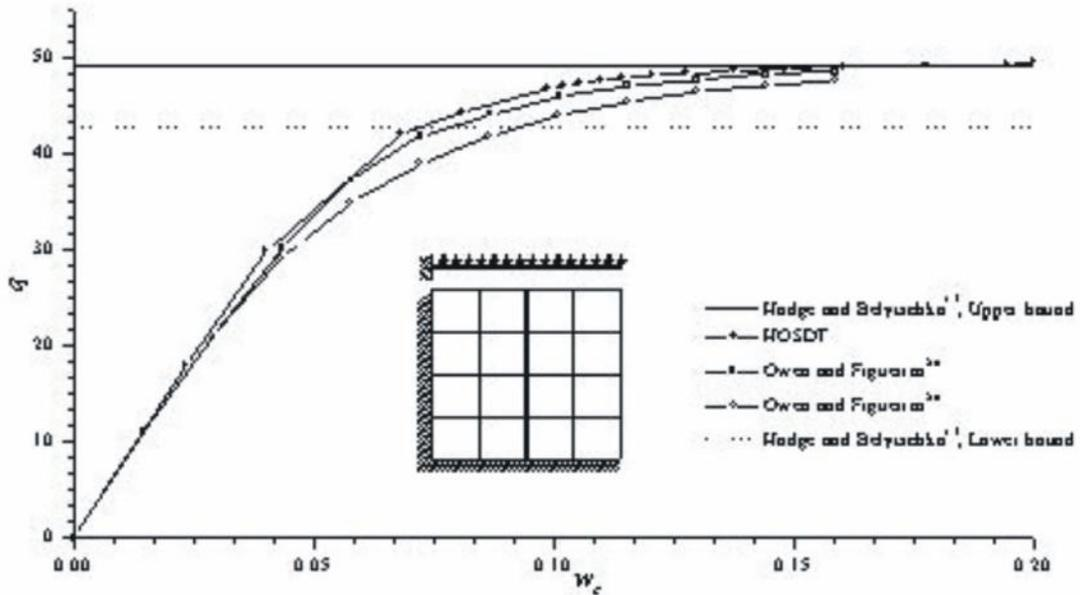
Fig. 4: Normalised load versus normalised central displacement for clamped circular plate with uniformly distributed load: Comparisons of different formulations for  $a/h=30$
