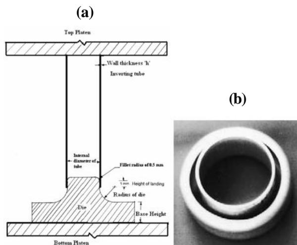
Fig. 1: (a) Experimental set-up used for performing external inversion of different round tubes; (b) Photographic view of typical inverted tube
