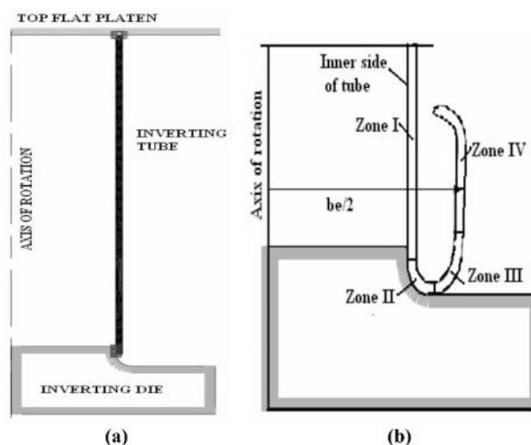
Fig. 3: (a): Proposed Computational Model, (b): Division of deformed profile into four zones of interest
