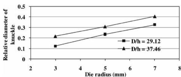
Fig. 5: Variation of relative diameter of knuckle with radius of die for different specimens
