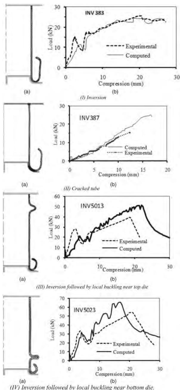
Fig. 2: Different (a): modes of deformation with their corresponding; (b): load-compression variations, which may occur during the external inversion of thin-walled tubes over a die
