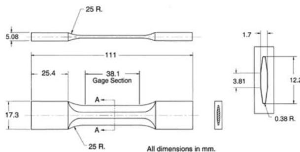
Fig. 1: Geometry of the leading edge test specimen and cross section dimension for FEM simulation [17]
