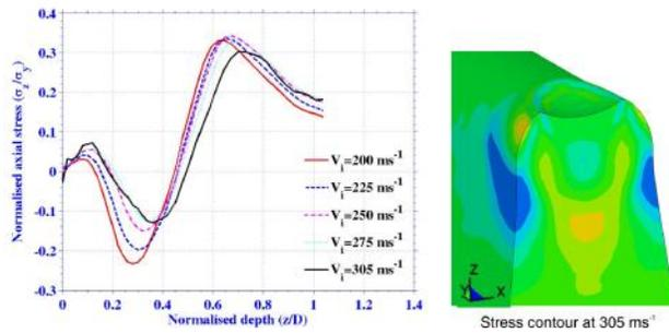
Fig. 6: Variation of residual axial stress ( $\sigma_z$ ) at different velocities
