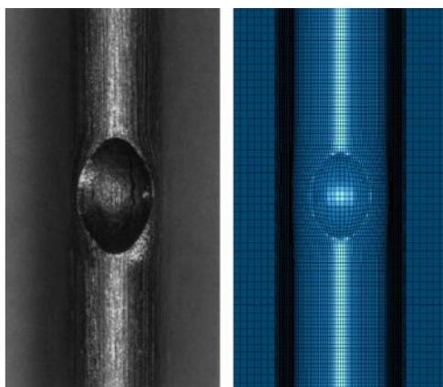
Fig. 3: Comparison of crater shape FEM analysis with test results [22]
