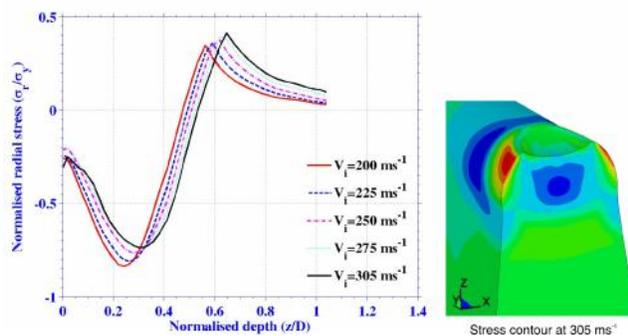
Fig. 7: Variation of residual axial stress ( $\sigma_y$ ) at different velocities
