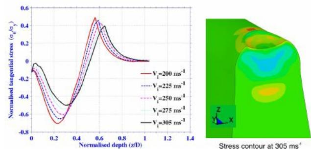
Fig. 8: Variation of residual axial stress ( $\sigma_x$ ) at different velocities
