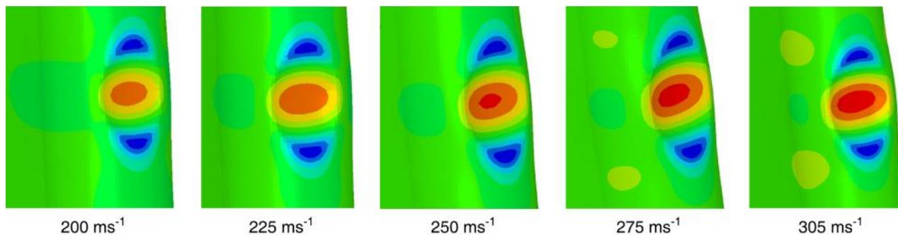
**Fig. 9: Stress contour at different projectile speeds for axial load in FOD test specimen**
