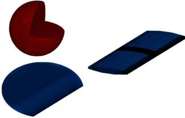
Fig. 2: Finite element model of spherical projectile and test specimen
