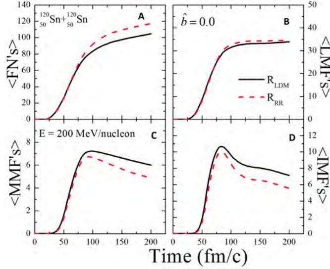
**Fig. 1: The time evolution of the mean multiplicity of (A) FN's [ $A = 1$ ], (B) LMF's [ $2 \leq A \leq 4$ ], (C) MMF's [ $5 \leq A \leq 9$ ] and (D) IMF's [ $5 \leq A \leq 40$ ] for the reaction of  ${}_{50}^{120}\text{Sn} + {}_{50}^{120}\text{Sn}$  at an incident energy of 200 MeV/nucleon for central collisions**
